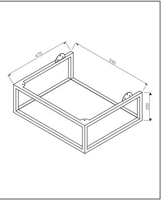
Dimensions (measurements in mm)
