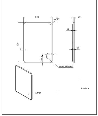
Dimensions (measurements in mm)
