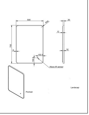
Dimensions (measurements in mm)
