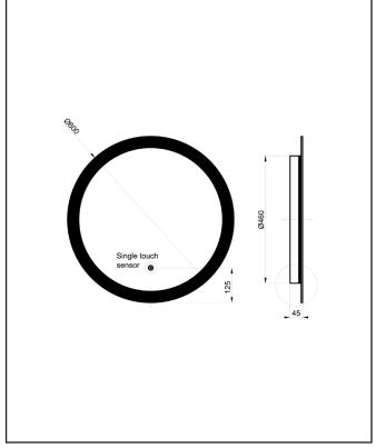
Dimensions (measurements in mm)
