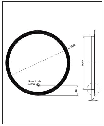
Dimensions (measurements in mm)
