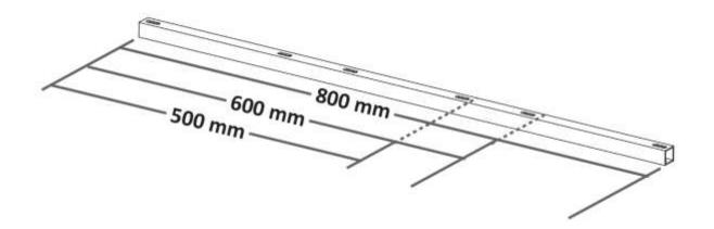
2. Attach the support bars to the frame and screw into place.
