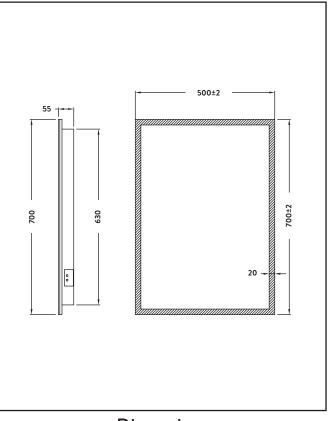
Dimensions (measurements in mm)
