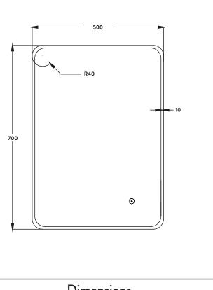
Dimensions (measurements in mm)
